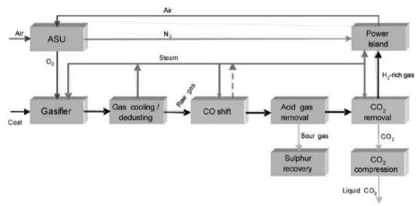
Figure 4: Pre-combustion CO<sub>2</sub> capture [7]
