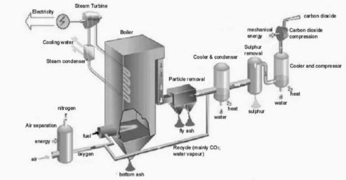
Figure 3: Oxyfuel combustion scheme (Vattenfall)
