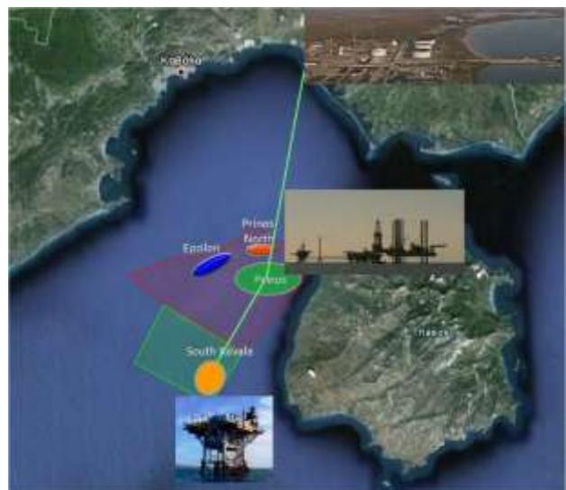
Kappa, built for the exploitation of the South Kavala gas field, an 8 leg processing platform Delta which includes a three phase separation process, crude dehydration, oil pumping, sour gas dehydration, produced water treatment, water injection, sweet gas-lift, and other auxiliary facilities.
