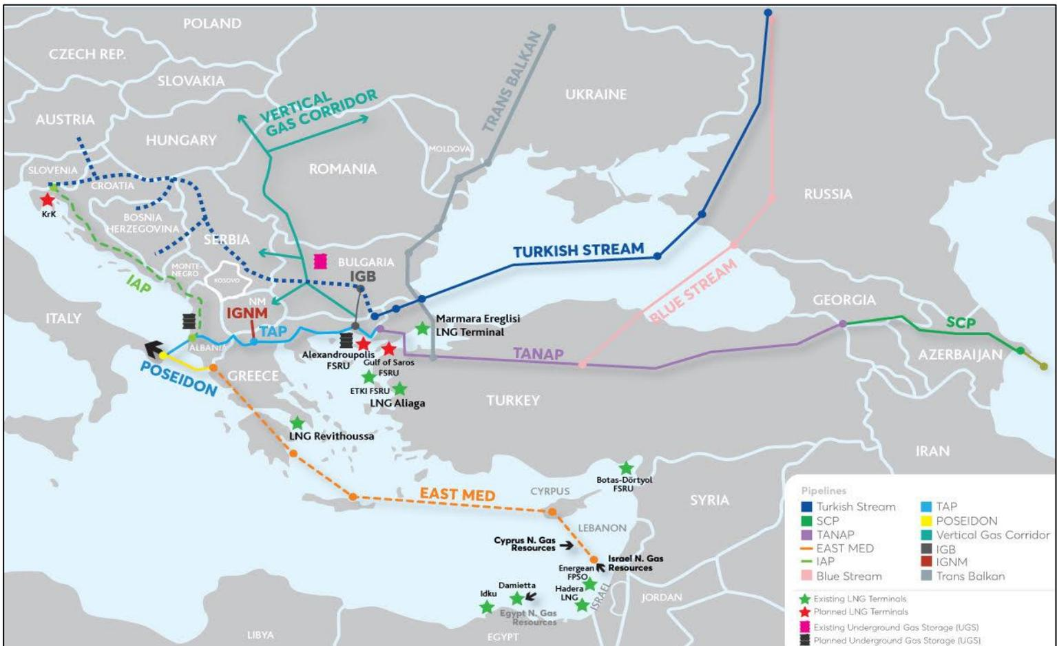
NB.: The TANAP has been completed, while TAP, Turkish Stream, BRUA and IGB are under construction. The IAP, the IGI Poseidon in connection with East Med pipeline and the Vertical Corridor and the IGF are still in the study phase. Blue Stream and Trans Balkan are existing pipelines.
