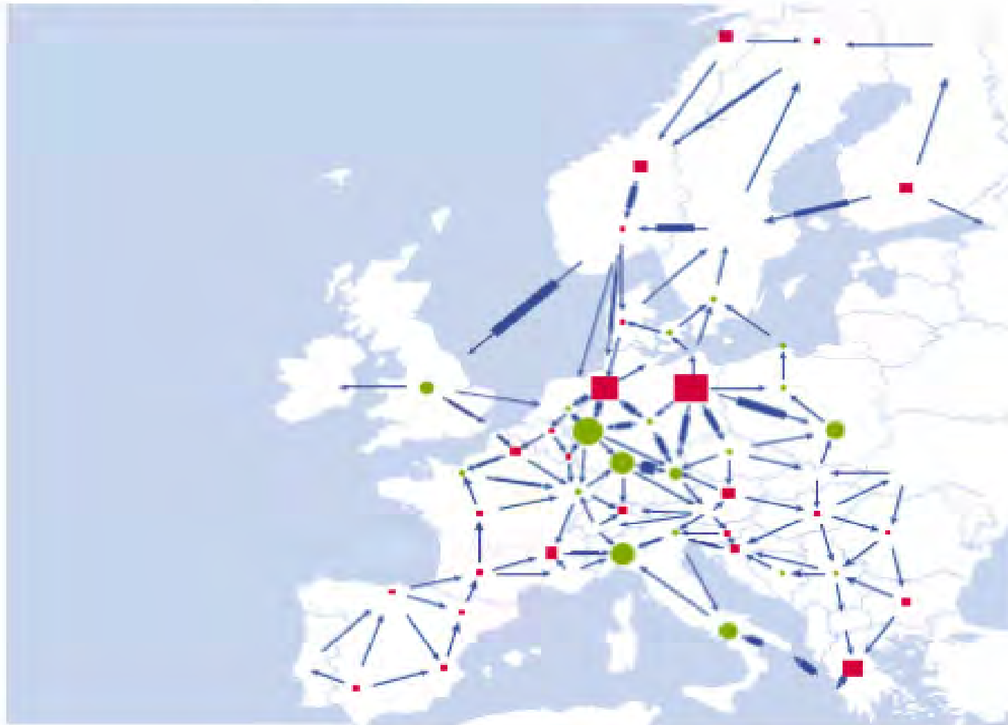
FIGURE [17]: Change in net energy flow in 2030 due to Stage 2 reinforcements. Green circles: Reduction in production. Red squares: Increase in production.
