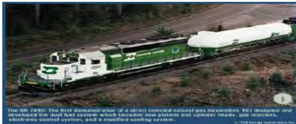
Locomotive converted to LNG, US
