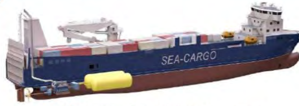
LNG powered vessel design (source: DNV)
