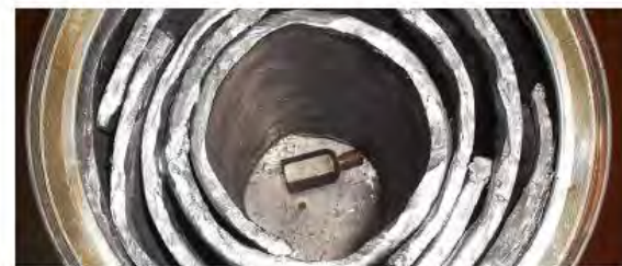
In the absence of an appropriate lead container, the source was placed in an “internal container” that was engineered with available materials and with layers of lead. (Photo: IAEA)
