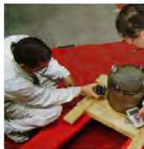
Fig. 2: Measuring dose rate of a sealed radioactive source
