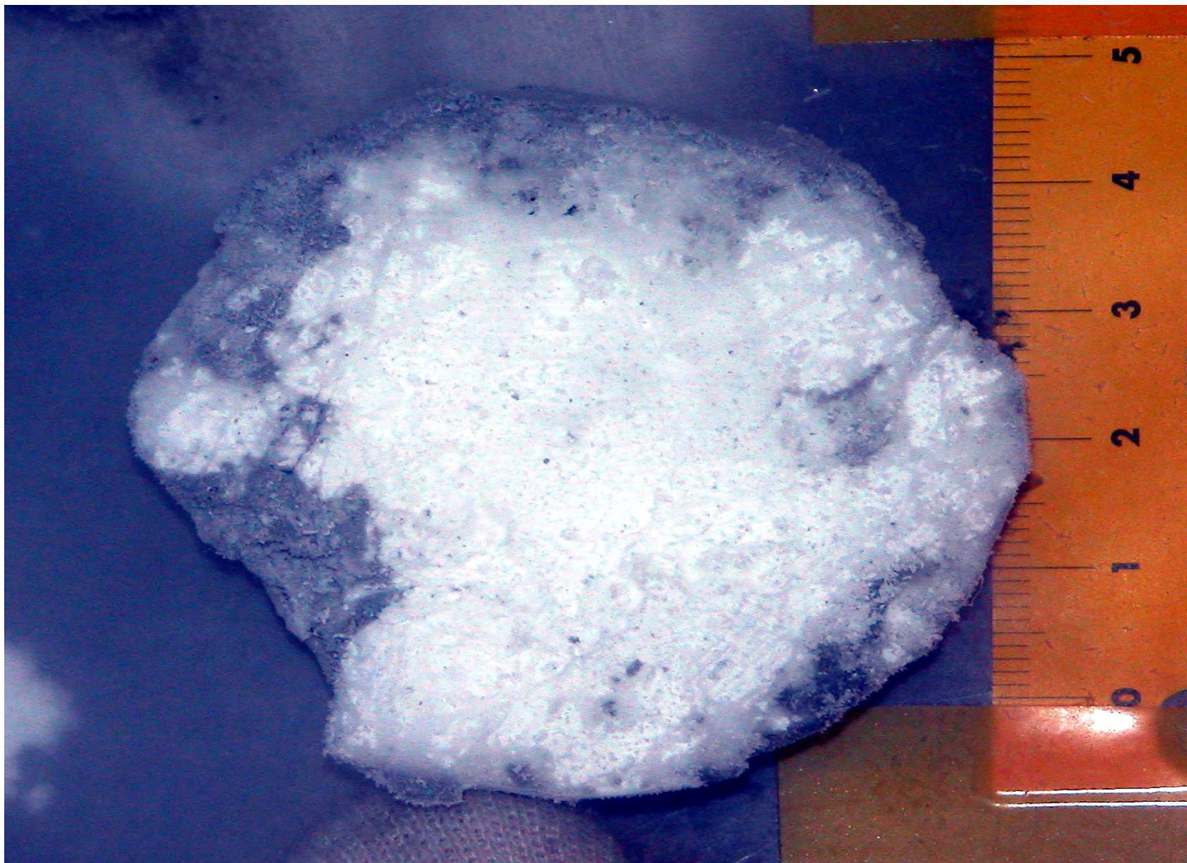
Figure 10. Hydrate from the Thessaloniki mud flow volcano of Anaximander mountains, Eastern Mediterranean, Lykousis et. al., 2004.
